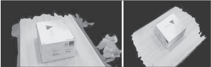
Fig. 4. A model created from 250 photos (on the left) and the modified model (on the right) (Czakóová & Takáč, 2020)
